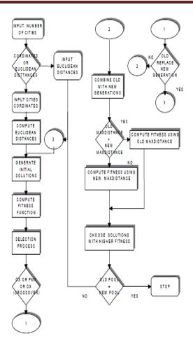
Fig: 3. The Flow Diagram For TSP Using GA Software System
