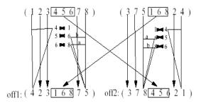
First, it selects uniformly at random two cut points along the strings, which represent the parent's tours. The sub strings between the cut points are called the mapping sections. In the above example they define the mapping 4-1, 5-6, and 6-8. Now the mapping section of the first parent is copied into the second offspring and the mapping section of the second parent is copied into the first offspring.
